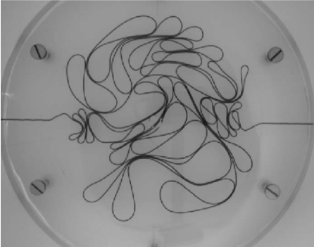
FIG. 1. A real packing configuration of no. 19AWG copper wire within the cavity of 20.0 cm of diameter.
